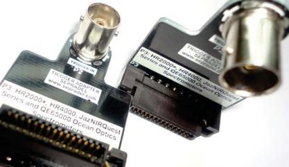
Our adapter, model OOTRIGGER, brand Sepradel® allows access to Trigger Signal of Ocean Optics Spectrometers; While providing a BNC connector for a standard coaxial line. The Sepradel® Trigger Adapter is compatible with the following Ocean Optics spectrometers:
